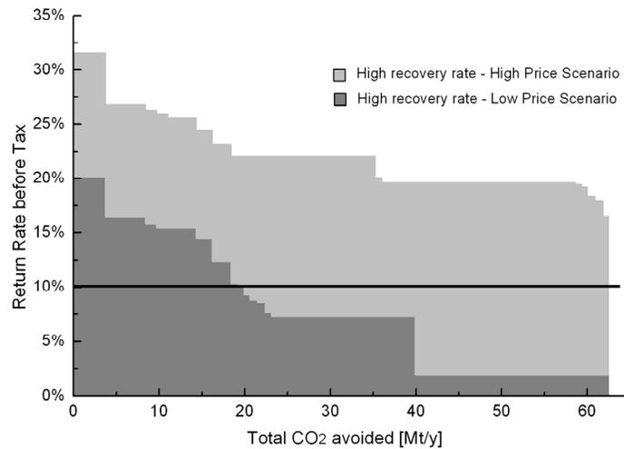
Figure 1: Cumulative CO<sub>2</sub> avoided by CO<sub>2</sub>-EOR for the 15 fields coming close to depletion, depending on the acceptable project return rate for realisation. High incremental oil recovery.
