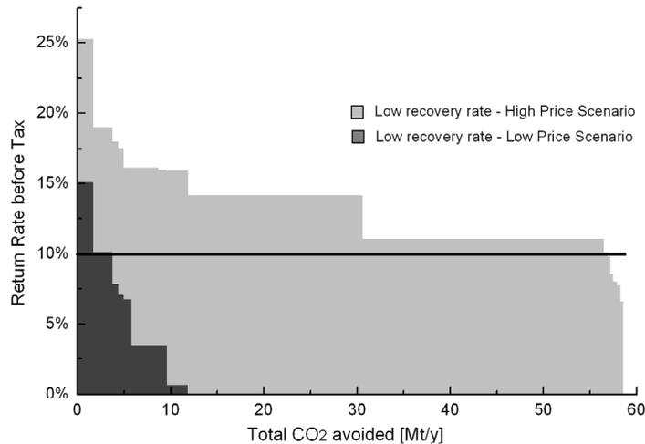
Figure 2: Cumulative CO<sub>2</sub> avoided by CO<sub>2</sub>-EOR for the 15 fields, depending on the project return rate for realisation. Low incremental oil recovery.
