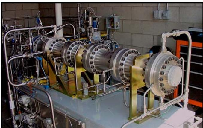
**Fig. 4:** The 20 MW<sub>i</sub> CES Gas Generator (GG). Combustor section is at far end followed by 4 sequential water-cooldown sections. Closest to observer is the downstream endplate that provided back-pressure during testing ‘in lieu’ of HP turbine.
